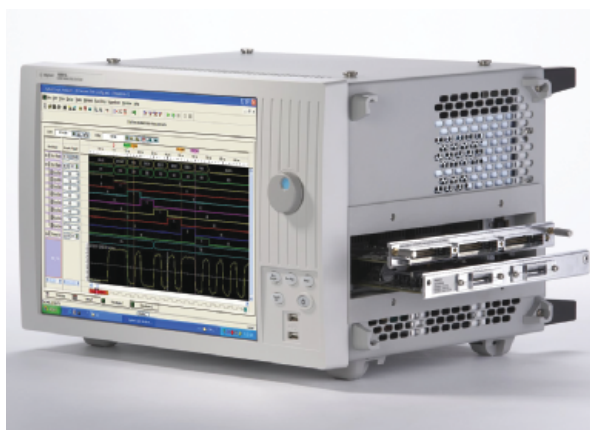
The two-slot, modular 16901A logic analyzer sports a 15-in. touchscreen display.
